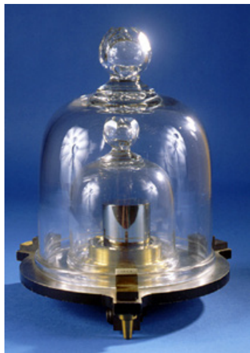
Figure 1.8 The Kilogram. The standard for the kilogram is a platinum-iridium cylinder kept in a special vault in France.
