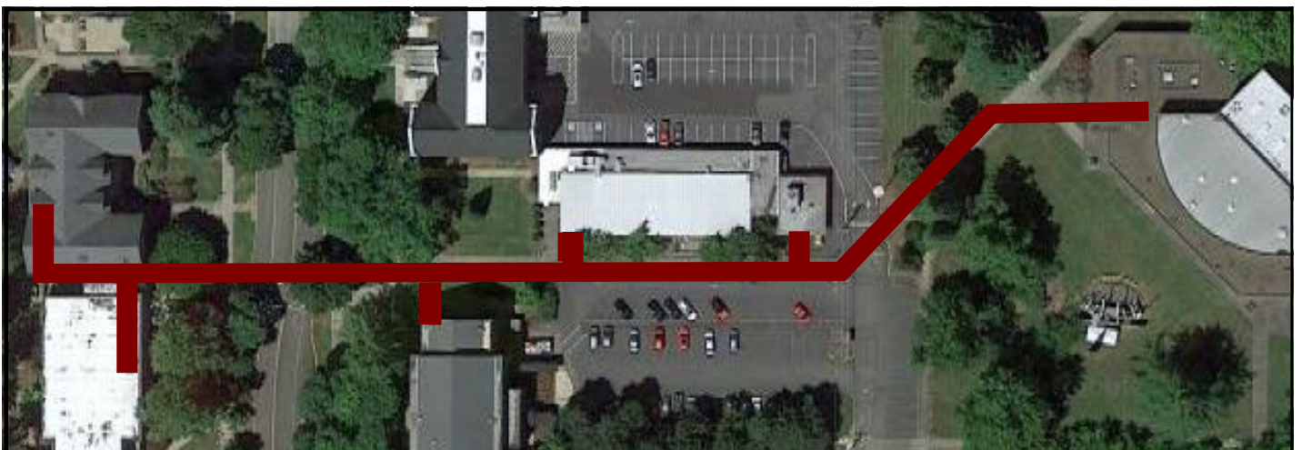
WOU tunnel system that carries the campus's fiber-optic lines, emergency power and other vital utilities
